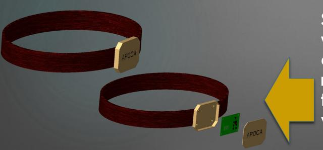
Sensor technology integrated into a wearable belt buckle that senses and detects objects in its line of sight – reports object distance-location back to the user via tone, vibration and or voice.
